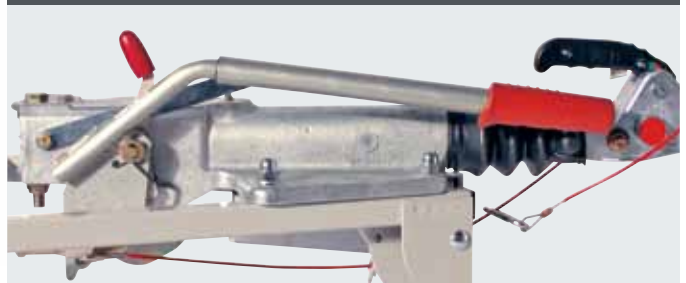
Hand brake lever opened = brake linkage not strained
