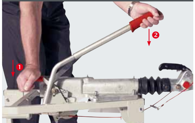
Hand brake lever tightened = brake linkage strained, hand brake lever lowered
