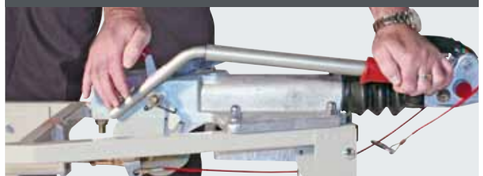
Hand brake lever tightened = brake linkage strained, hand brake lever lowered
