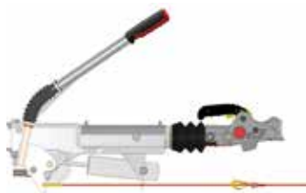
Handbrake lever applied (Position with trailer on down-slope)
